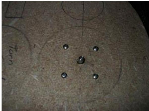
Drill a hole in the center of your gauge ring the same size as the hole for the motor shaft. Using the drill bit, center the plate over the hole as shown and drill the pilot holes for the mounting screws. Once the
