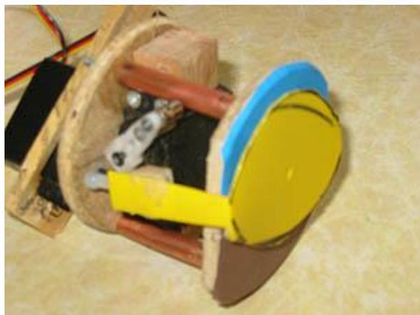
Having made the 'base', mount the second servo to it as shown in the picture to the left. Don't worry if it is not centered. We will address this later.
